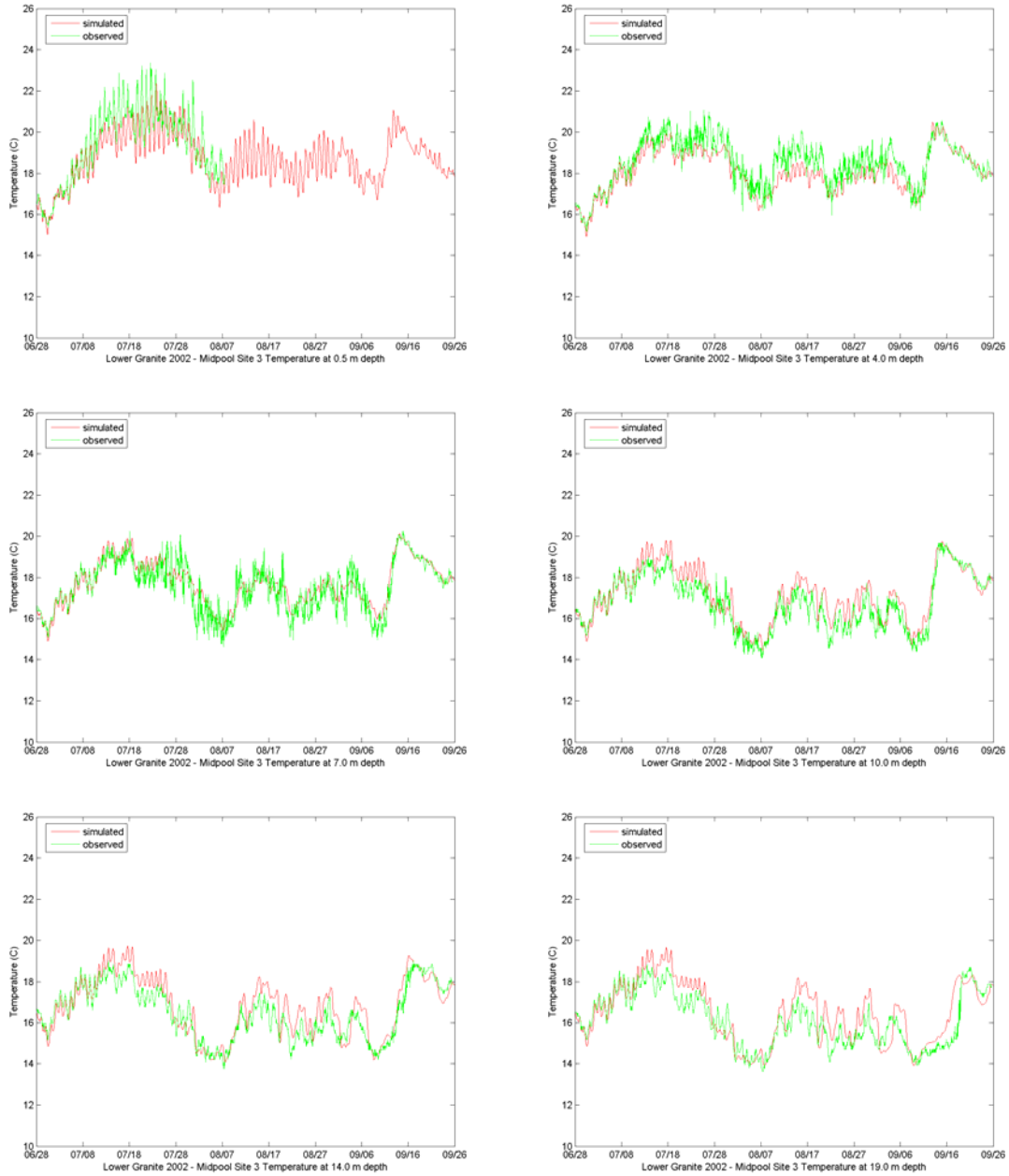
Figure C.3 Observed and Simulated temperatures at LWG Site 3, 2002
