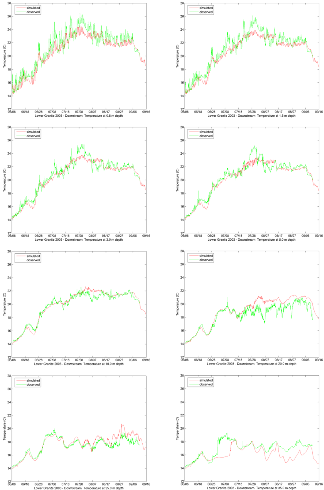
Figure C.11 Observed and Simulated temperatures at LWG Site 1, 2003
