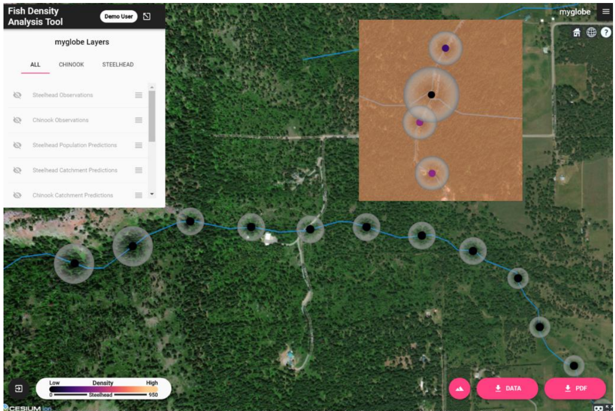
Figure 9. Prediction standard errors appear as translucent circles as the user zooms in. Circles are proportional to the relative magnitude of the standard error. The orange inset is simply an example showing differences in prediction standard errors from another part of the network.
