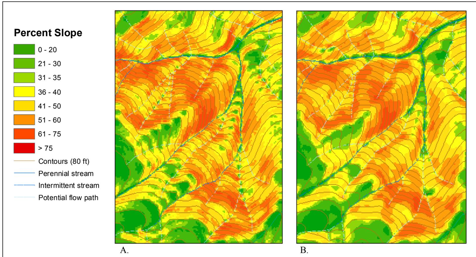
Figure 15. A comparison of slope values derived from (A) a standard USGS 10-meter DEM based on 7.5-minute elevation contours, and (B) a 10-meter drainage enforced DEM created at Redwood National and State Parks using TOPOGRID and the same base elevation data. Methods used at Redwood National and State Parks sought to minimize the contour biasing more evident in (A).
