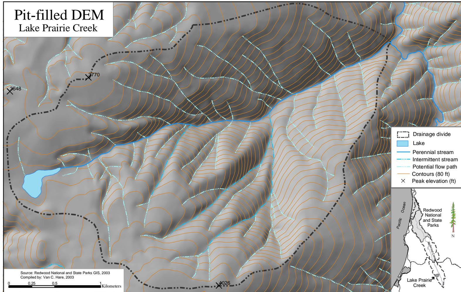
Figure 7. Lake Prairie Creek: shaded relief image of pit-filled DEM created at the beginning of the SHALSTAB modeling process. Also shown is the USGS hypsography (80 ft. interval), contour crenulated drainage network and peak elevation points used as input to the DEM creation process.
