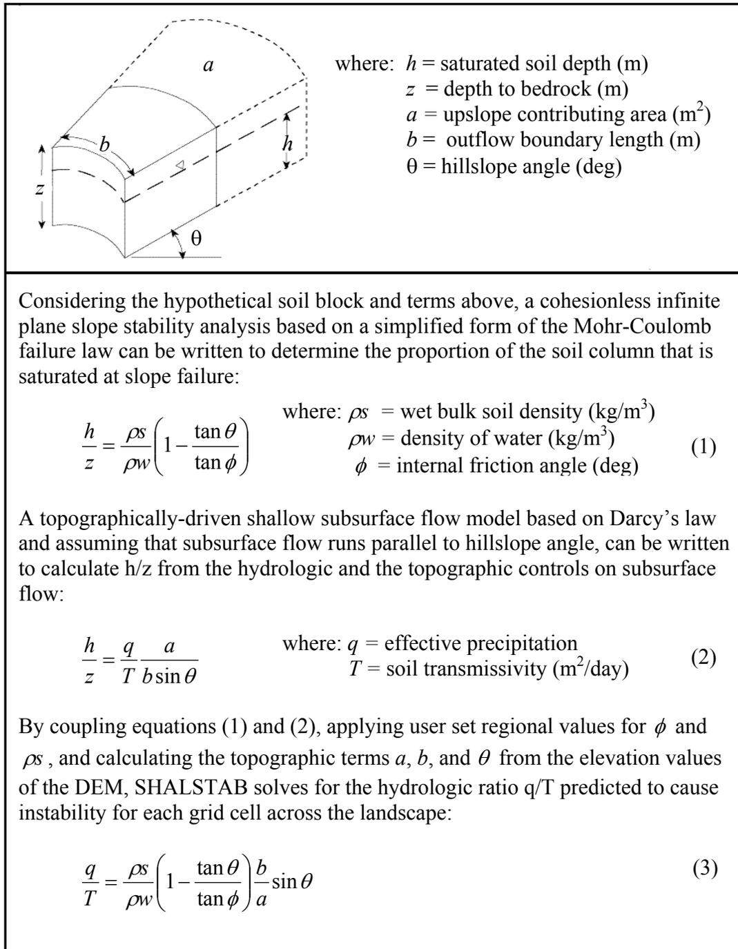
Figure 1. Diagram of partially saturated soil block and explanation of terms and assumptions used in the SHALSTAB model (Dietrich et al. 2001, diagram after Schaub 1999).
