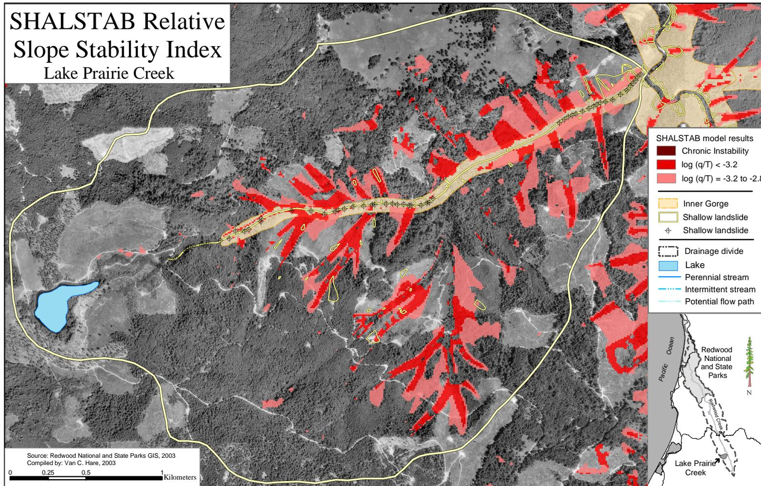
Figure 11. Lake Prairie Creek: final  $\log(q/T)$  grid resulting from SHALSTAB model run where  $\phi = 45$  and  $p_s = 1700 \text{ kg/m}^3$ . Slope ( $\theta$ ) is determined from the slope grid presented in Figure 8, and  $a/b$  is determined from the flow accumulation grid presented in Figure 10. Also shown is the inner gorge and the shallow landslides used for model validation.
