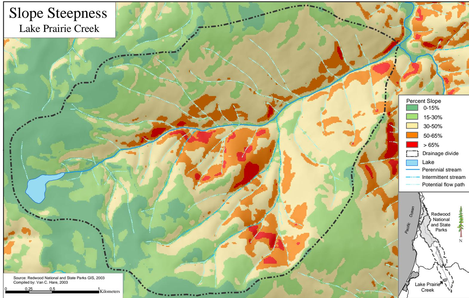
Figure 8. Lake Prairie Creek: slope grid created by SHALSTAB (step 3) based on the pit-filled DEM presented in Figure 7. Slope calculation methods are as described by Dietrich and Montgomery (1998).
