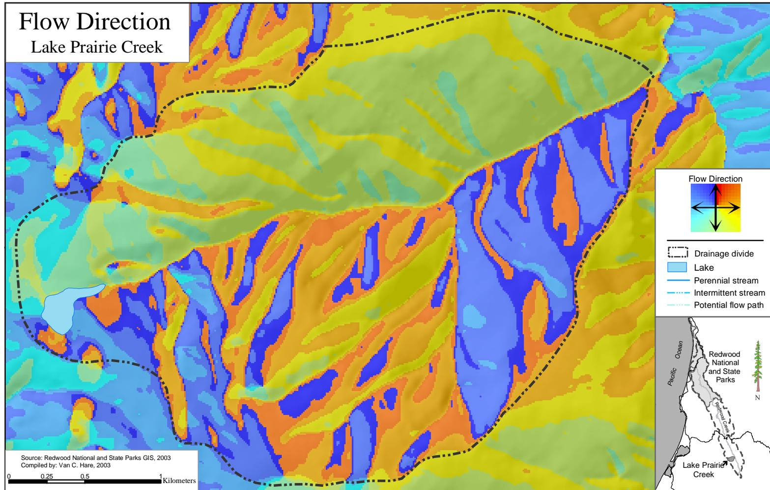
Figure 9. Lake Prairie Creek: flow direction grid created by SHALSTAB (step 4) based on the pit-filled DEM presented in Figure 7. Flow direction calculation methods are as described by Dietrich and Montgomery (1998).
