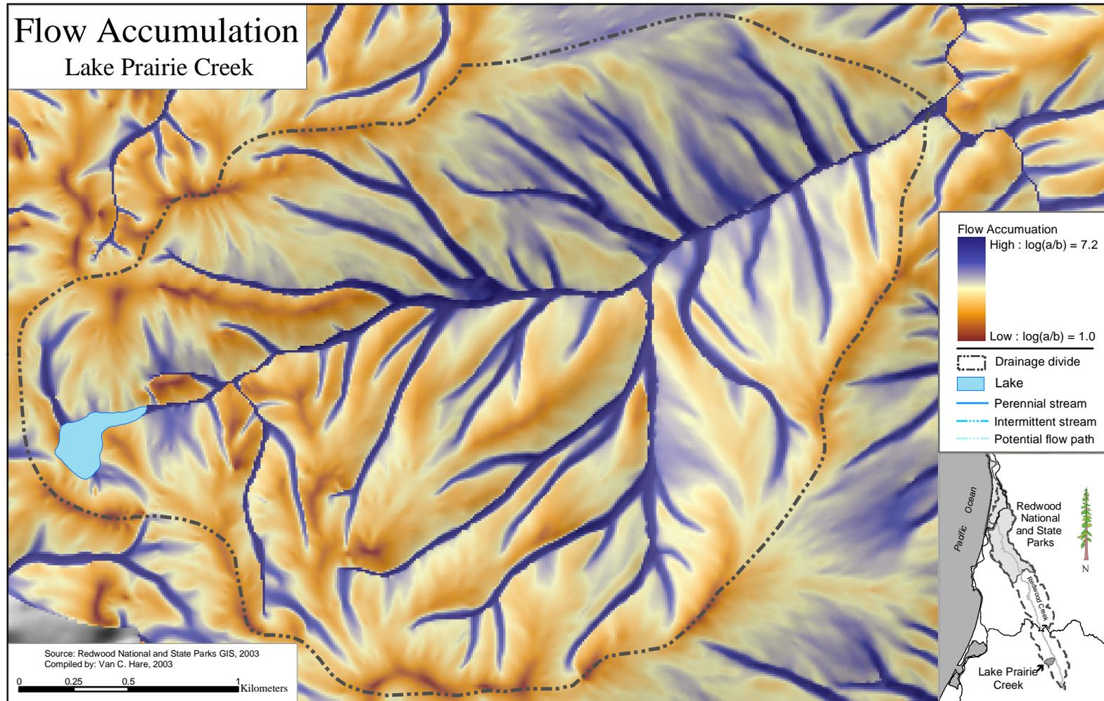
Figure 10. Lake Prairie Creek: flow accumulation grid created by SHALSTAB (step 5) based on the flow direction grid presented in Figure 9. Flow accumulation indicates the specific catchment area ( $a/b$  or upslope contributing area / grid cell size) for each cell. It is displayed here on a log scale.
