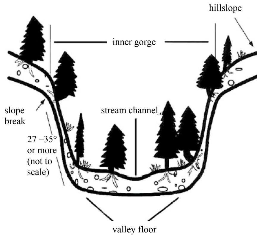
Figure 5. Diagram of an inner gorge, emphasizing the abrupt steepening below the break in slope (after Washington Forest Practices Board, 2000).
