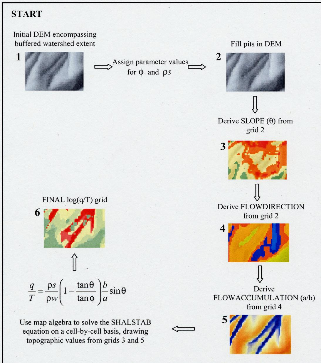
Figure 6. Diagram outlining the SHALSTAB grid modeling process
