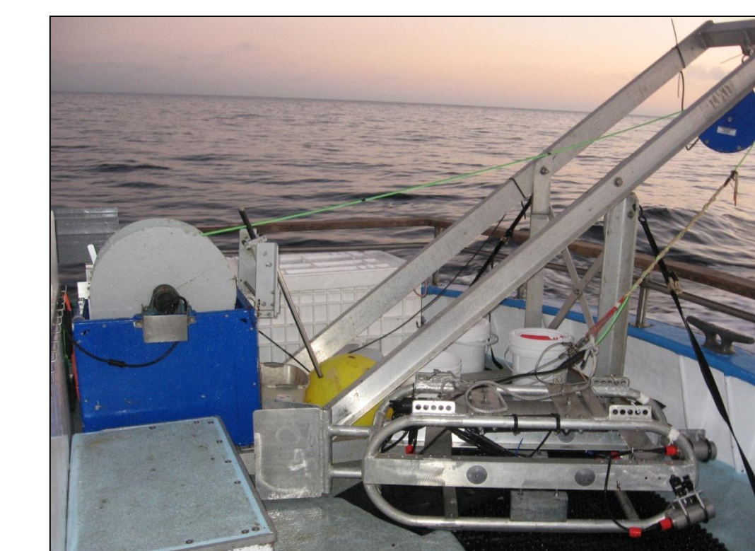
Figure 11. Custom-designed camera sled, winch, and A-frame as mounted on the F/V Aggressor.
