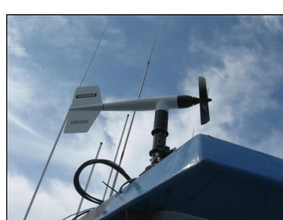
Figures 6a & b. Seabird 19plus CTD and anemometers record oceanographic and weather conditions during each sampling event.
